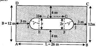
There are two rectangles ABCD and EFGH and two semicircles EHI and GFJ. For dimensions of shapes,
